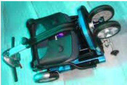
Pull down the tiller to fold the scooter.
